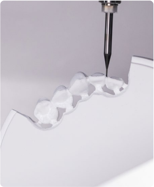
The E5 machines anterior teeth at a 90° angle. The tool, guided perpendicular to the vestibular surface, reduces residual material while improving surface quality.
